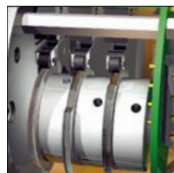
Switch cam with configurable "switching patterns"
